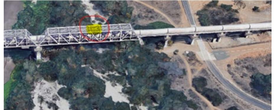
Upper Feeder bridge crossing with identifying location of the temporary solar-powered generator
