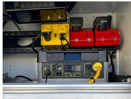
Components of the solar generator fitted to a work truck. From left to right: battery inverter in the storage compartment, a close up of the Yeti battery inverter, and two 200-Watt solar panels on the back of the truck.
