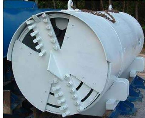
(d) Rotary cutting head w/ adjustable full face support (courtesy of Horizontal Equipment Manufacturing, Inc.)
