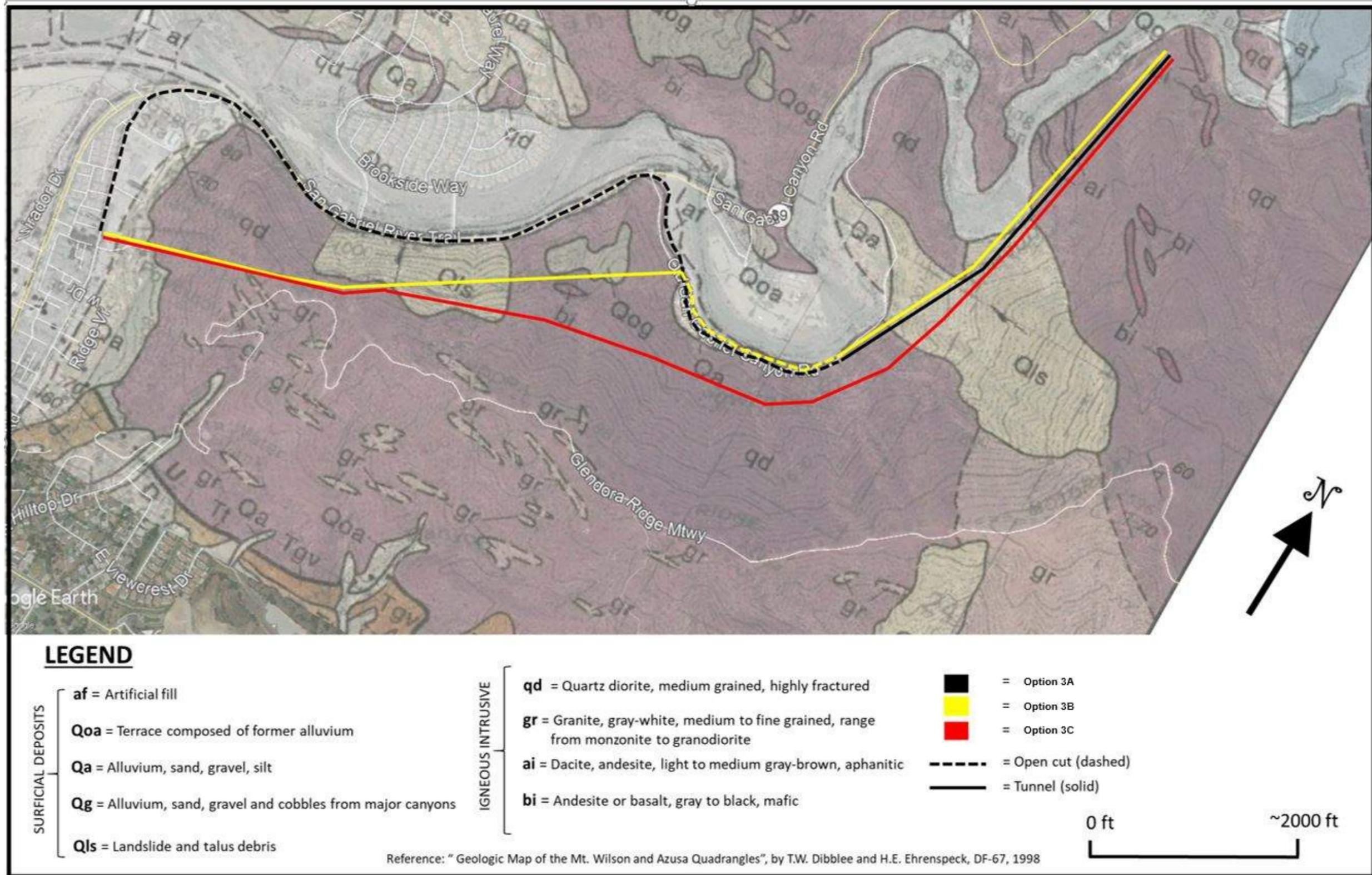
Figure 5-1. Geologic map Azusa-Glendora and proposed alignments, overlay on satellite photo
