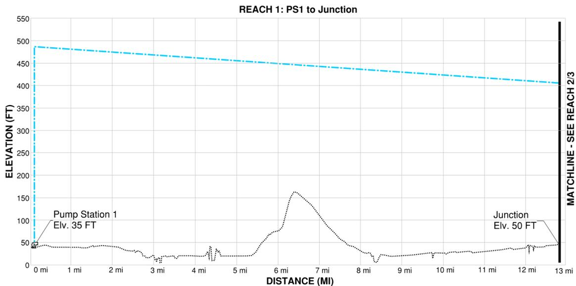
Figure 1-2 Reach 1 Hydraulic Profile (Alternative A)
