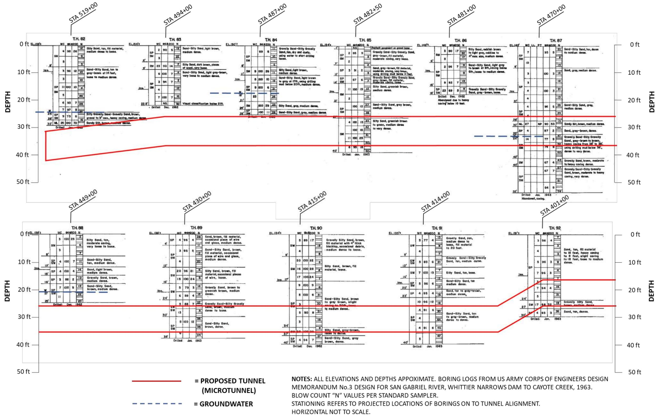
Figure 4-1. USACE logs with tunnel Sta. 519+00 to Sta. 401+00 and tunnel excavation profile
