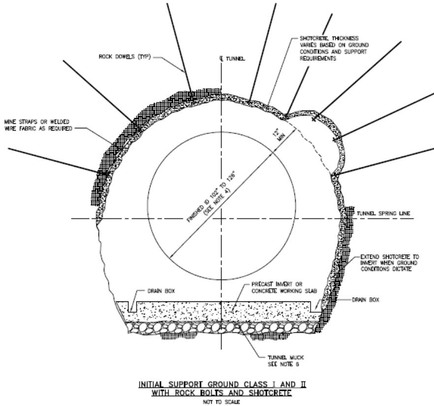
Figure A-10. Typical horseshoe-shaped drill-and-blast tunnel
