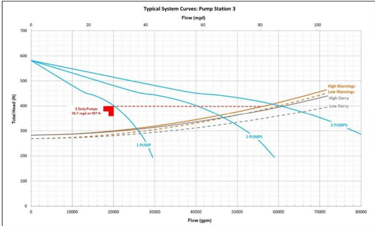
Figure 1-13 PS-3 System Curves (Alternative A and B)
