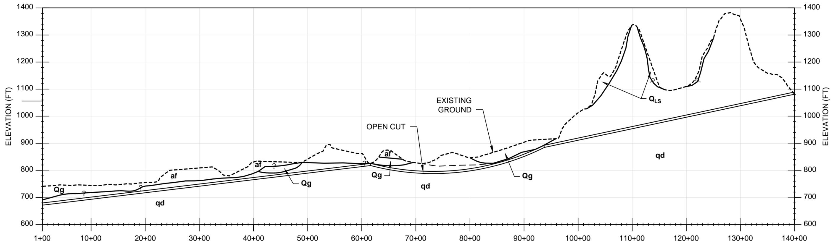
**FIGURE C9 - AZUSA TO GLENDORA OPEN CUT AND TUNNEL OPTION 3A**
