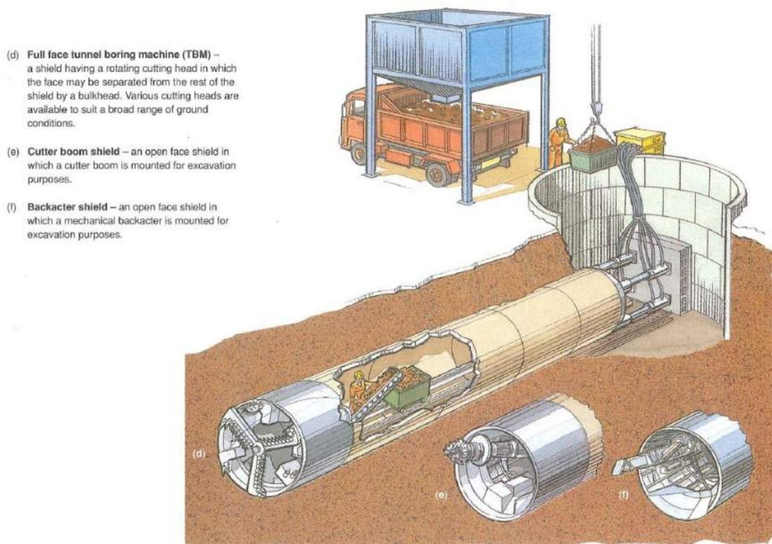
Figure A-3. Typical pipe jacking operation (PJA, 1995)
