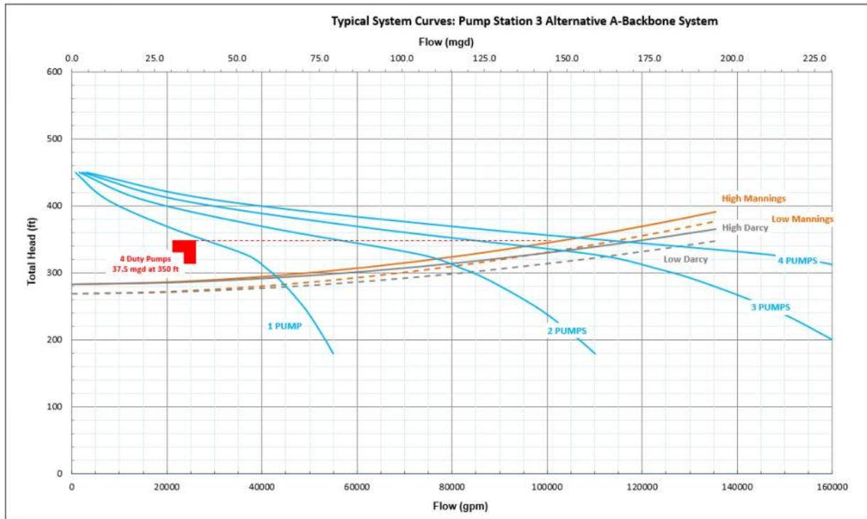
Figure 1-14 PS-3 System Curves (Alternative A-Backbone System)
