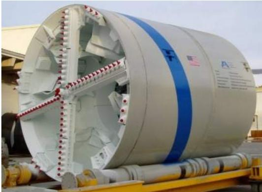
(c) Rotary cutting head w/ partial face support (courtesy of Akkerman, Inc.)
