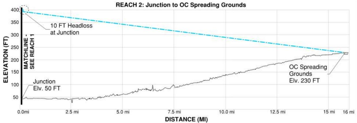
Figure 1-3 Reach 2 Hydraulic Profile (Alternative A)
