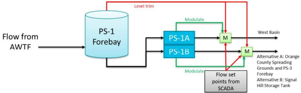
Figure 1-4 Flow Control with Level Trim and PS-1
