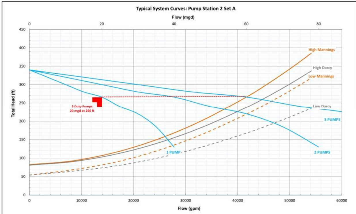
Figure 1-11 PS-2 Set A System Curves (Alternative B only)
