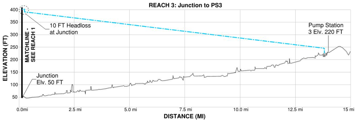
Figure 1-4 Reach 3 Hydraulic Profile (Alternative A)
