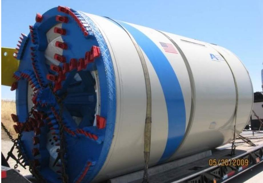
Figure A-7. Microtunnel boring machine
