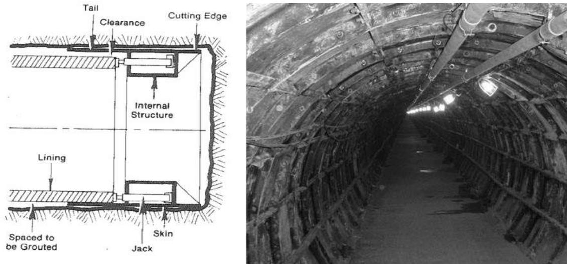
**Figure A-6. Conventional shield tunneling with liner plate support (Proctor and White, 1977)**
