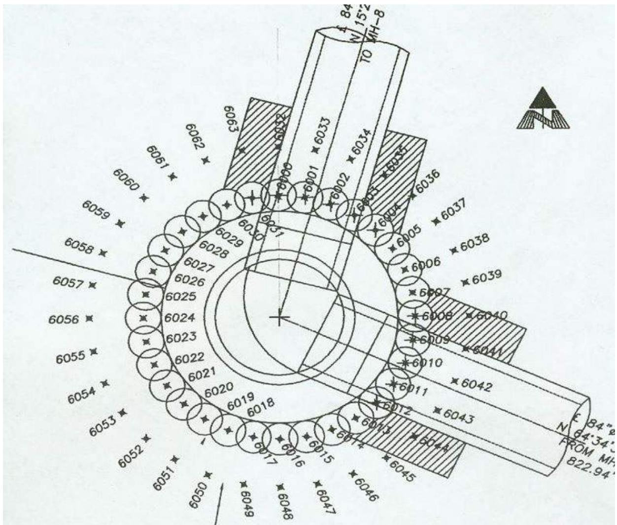
**Figure B-4. Typical secant pile shaft layout with overlapping concrete secant piles**
