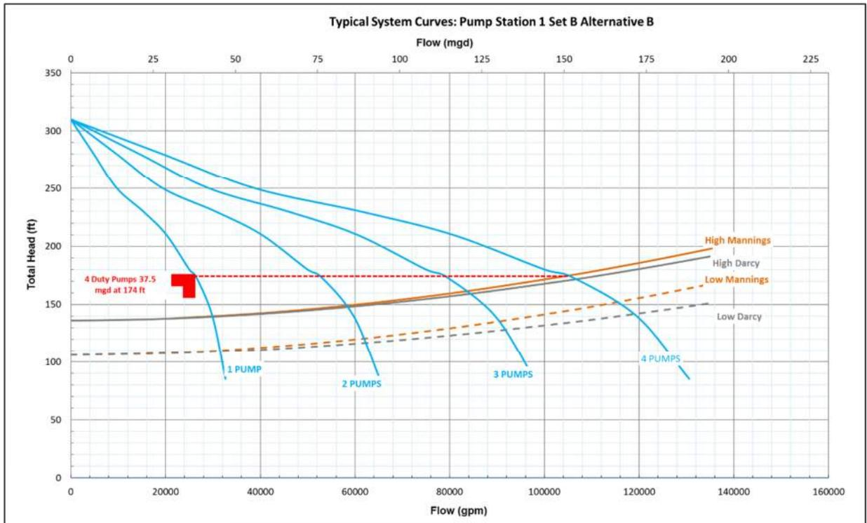
Figure 1-9 PS-1 Set B System Curves – Alternative B
