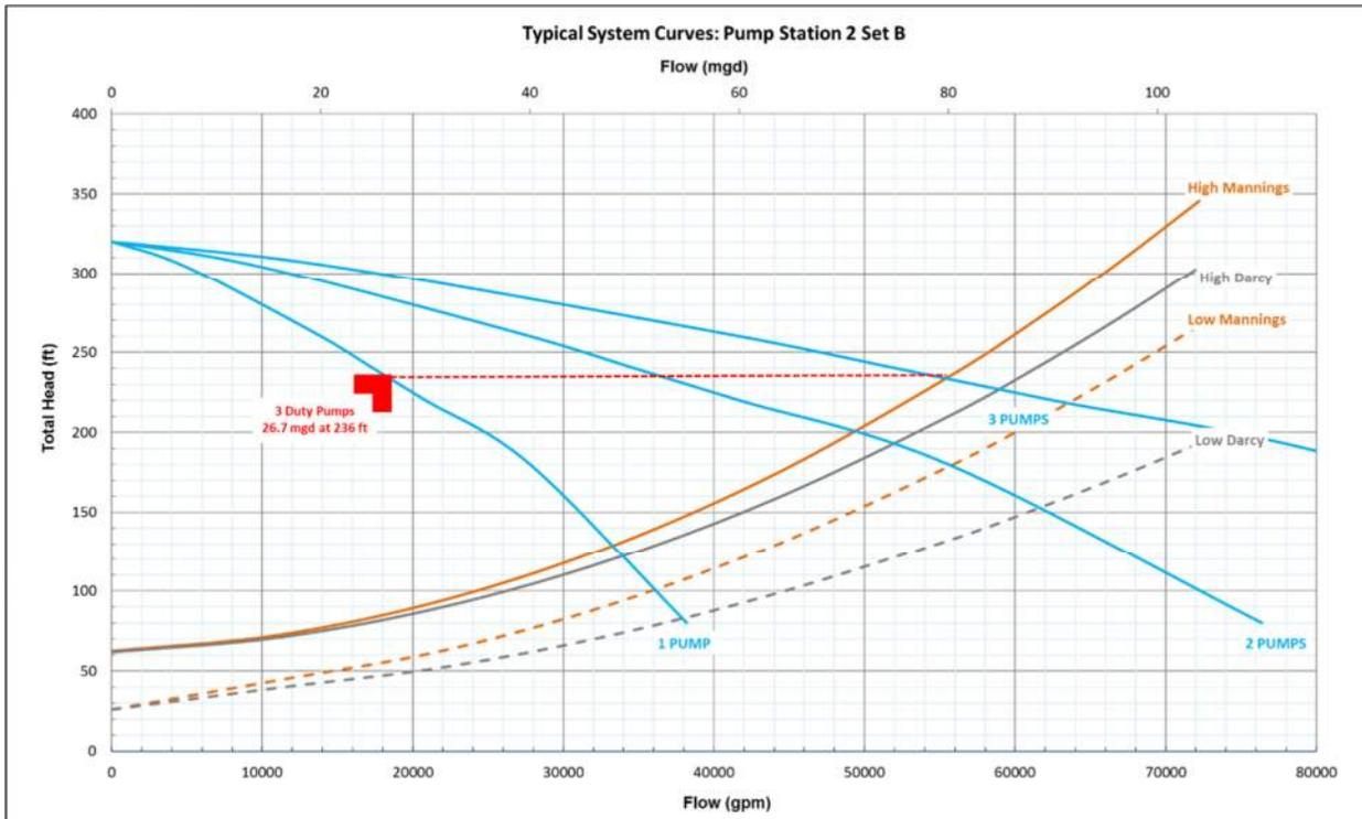
Figure 1-12 PS-2 Set B System Curves (Alternative B only)
