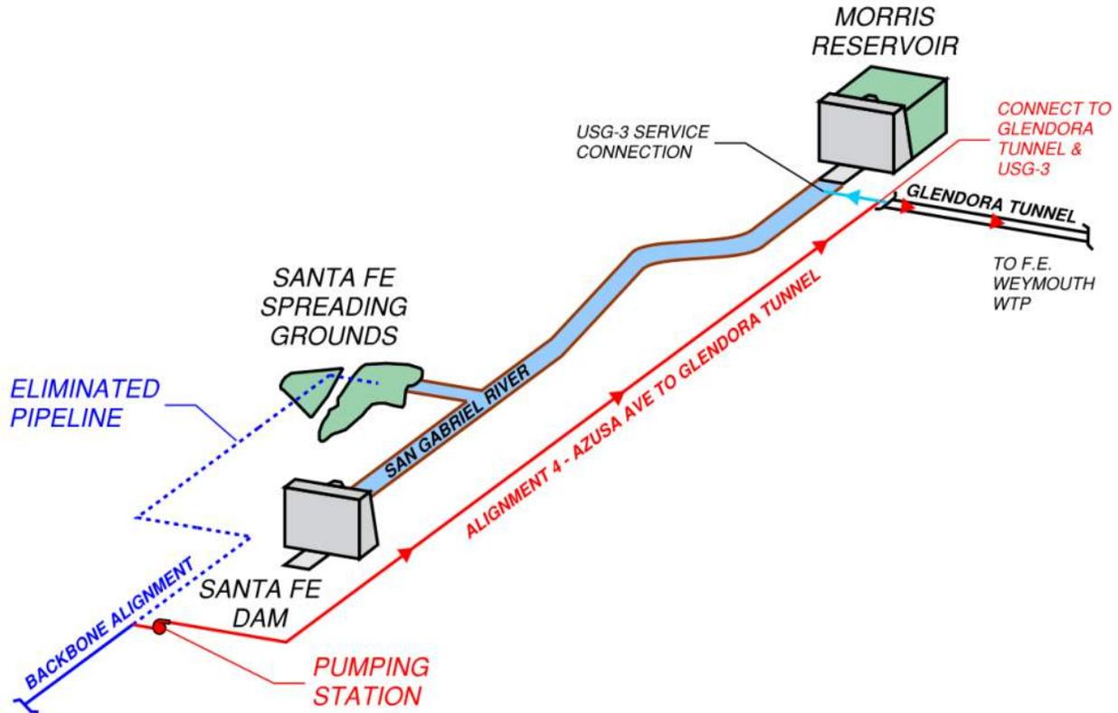
Figure 3-9 Alternative Discharge Location for Alignment 4 – Schematic View
