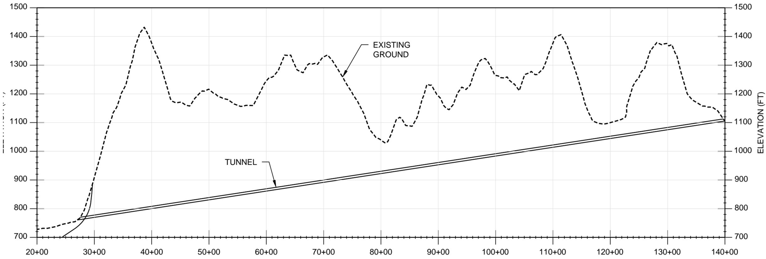
**FIGURE C11 - AZUSA TO GLENDORA - OPTION 3C - TUNNEL**
