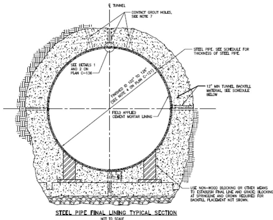
**Figure A-12. Typical horseshoe-shaped tunnel with the carrier pipe inserted and grouted in place**
