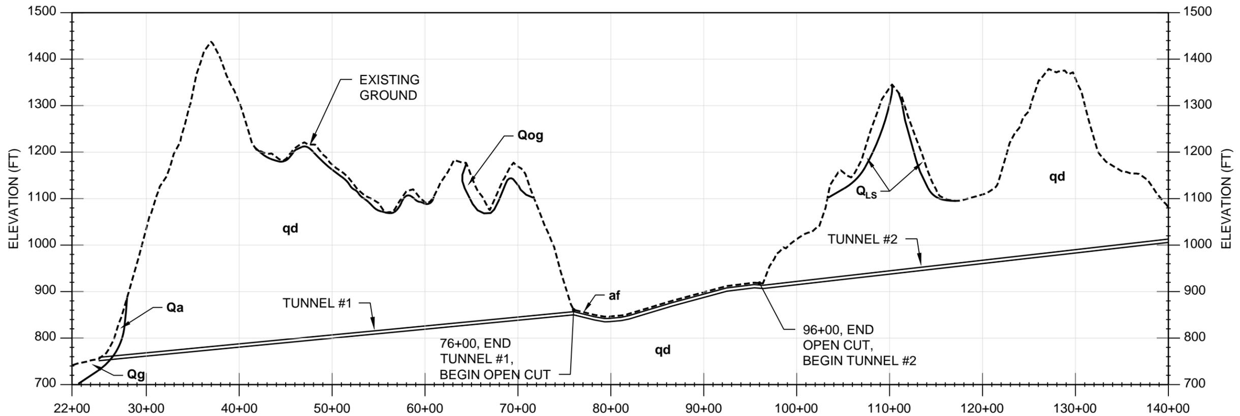
FIGURE C10 - AZUSA TO GLENDORA - OPTION 3B - TUNNEL-OPEN CUT-TUNNEL
