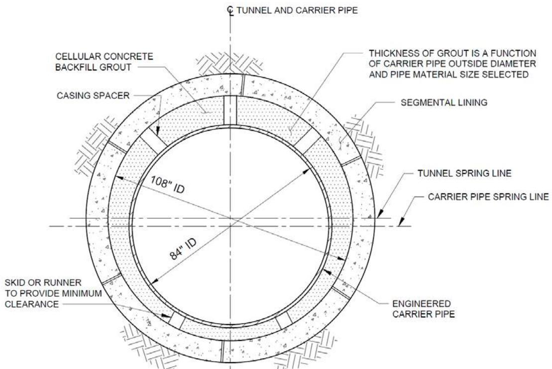
**Figure A-2. Typical initial tunnel lining and carrier pipe configuration for tunneling**
