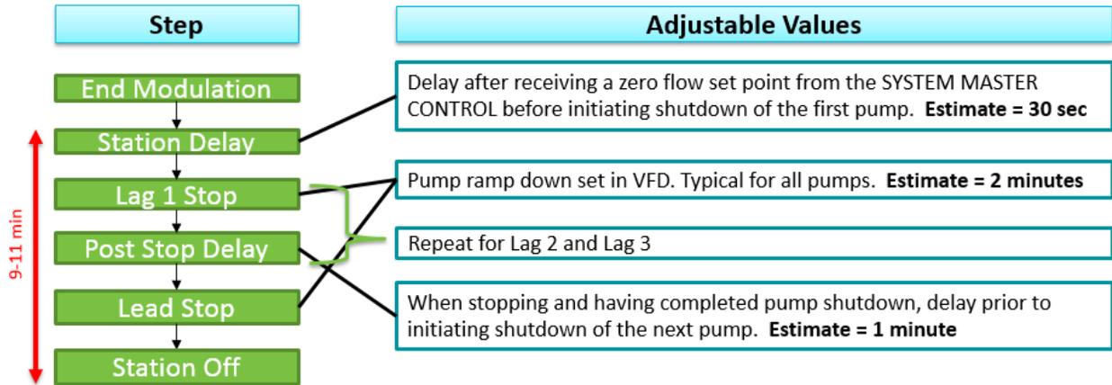
**Figure 1-6 Conceptual Stopping Sequence**
