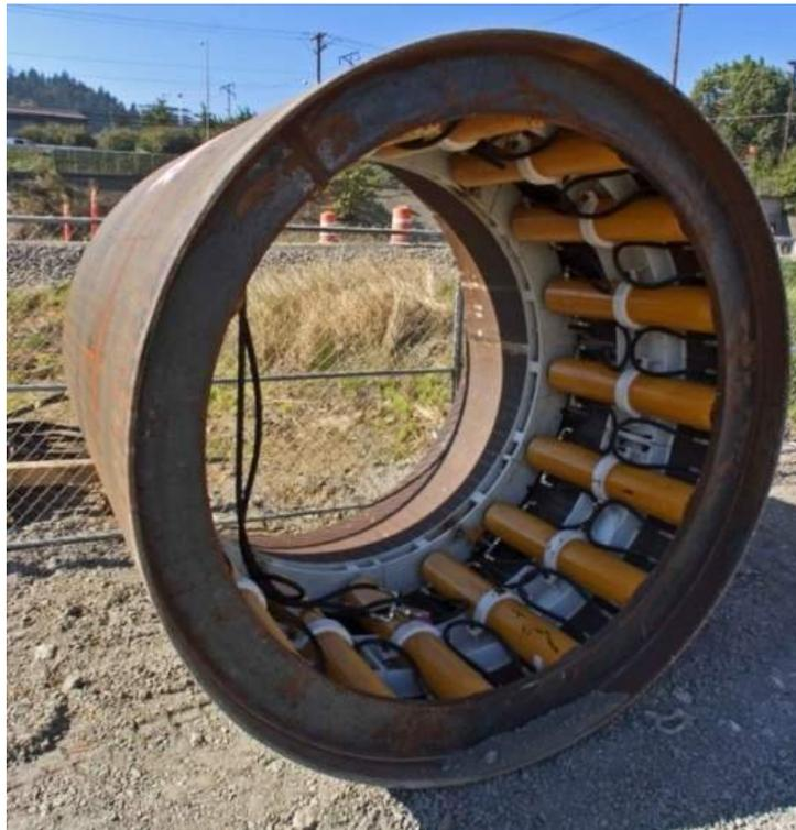
**Figure A-4. Intermediate jacking station**
