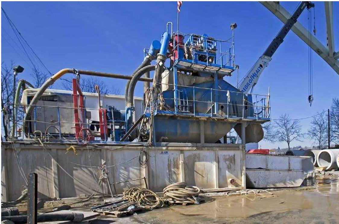
**Figure A-9. Typical slurry separation plant setup**
