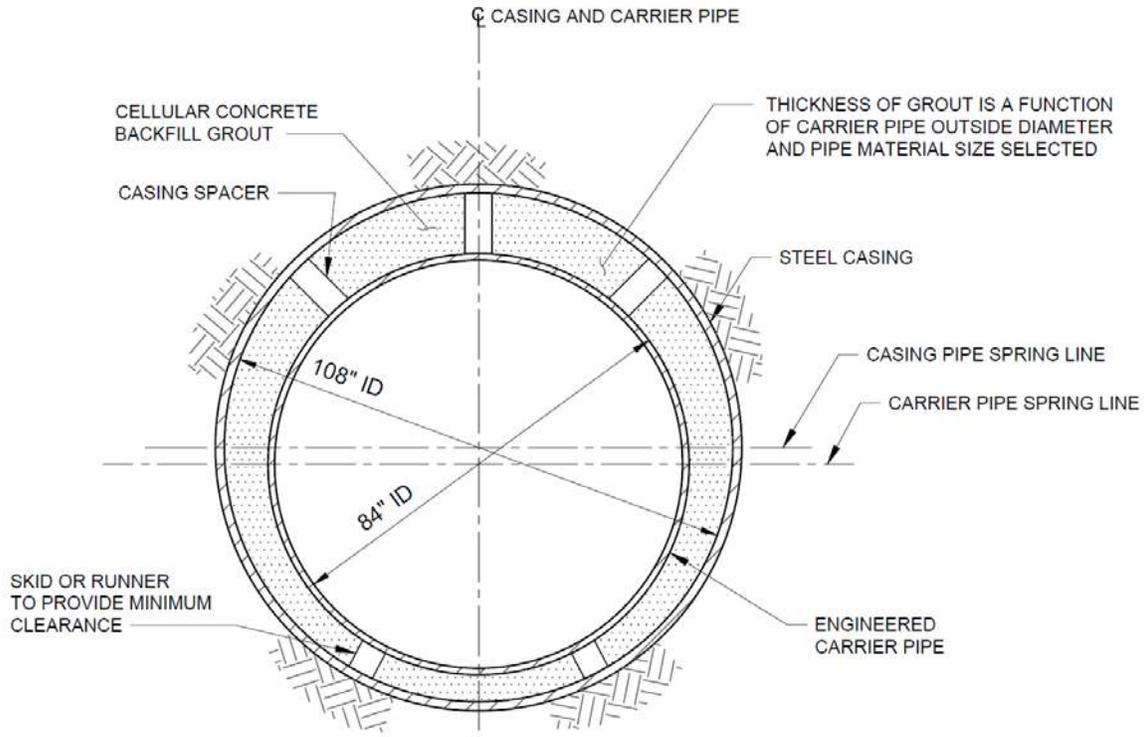
**Figure A-1. Typical casing and carrier pipe configuration for pipe jacking and microtunneling**
