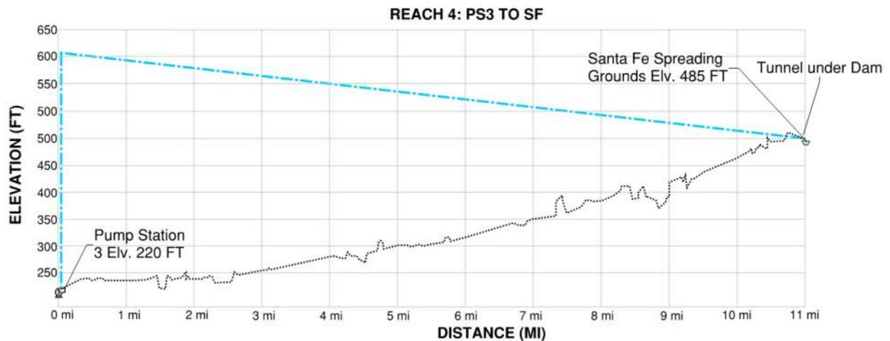
Figure 1-5 Reach 4 Hydraulic Profile (Alternative A)
