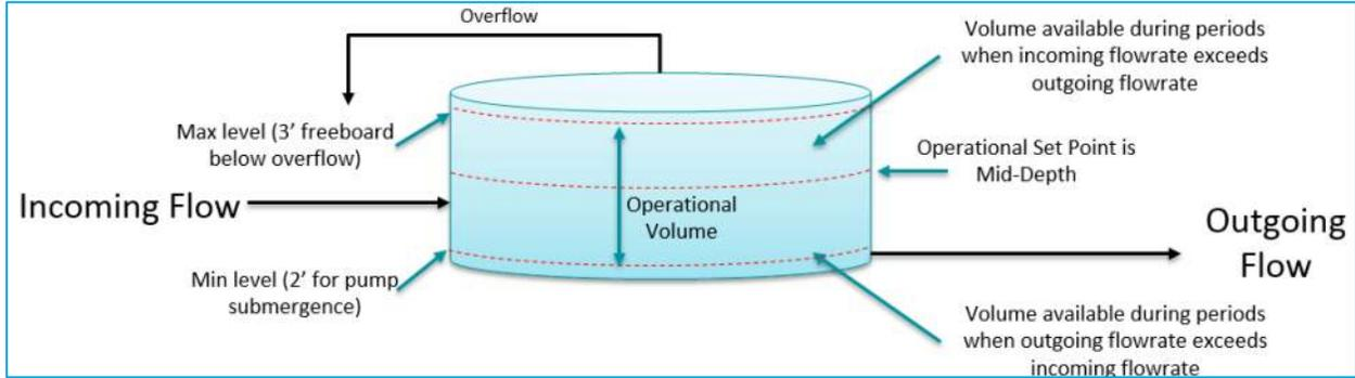
**Figure 1-16 Typical Tank Level Configuration**
