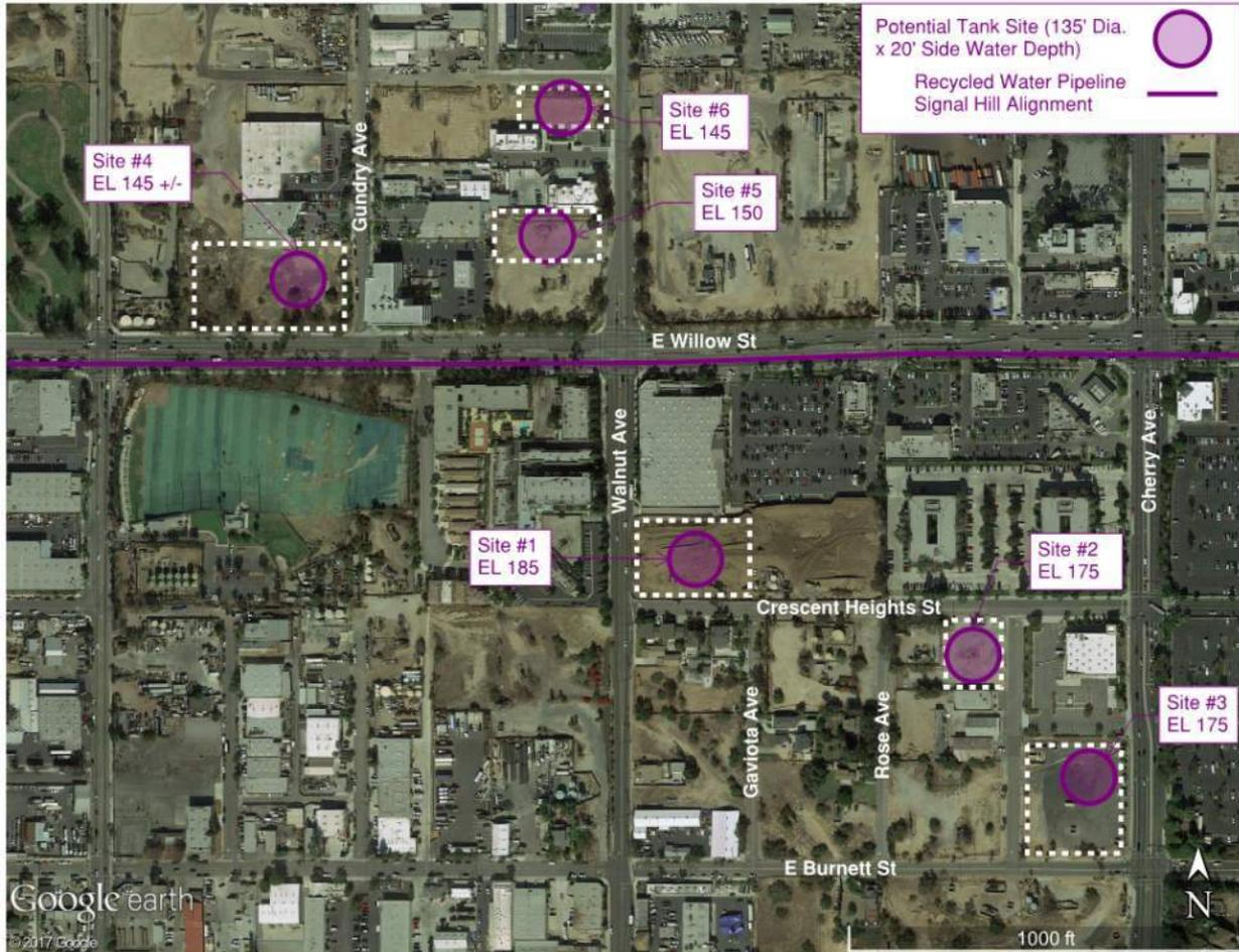
Figure 3-1: Signal Hill Tank Location Map
